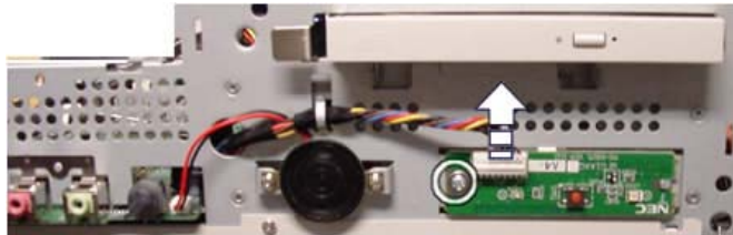
Fig. 20: Removing the Switch/LED board
